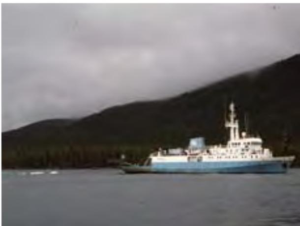
*The R/V Maurice Ewing in British Columbia towing airguns that fire incrementally recording a seismic image profile.*
