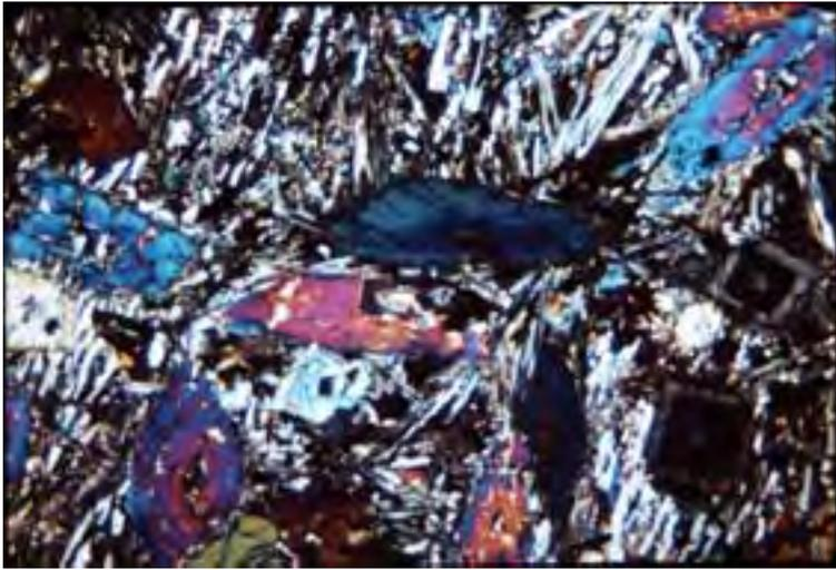
*Photomicrograph of a thin section of lunar basalt, collected by the Apollo 12 mission. This texture of sector-zoned pigeonite clinopyroxene phenocrysts and swallowtail plagioclase is produced by rapid cooling of the source magma at the surface of the Moon.*
